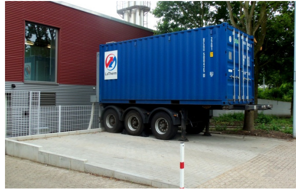
Figure 23: Trailer with a container and a latent heat storage system (Source: LaTherm GmbH)
