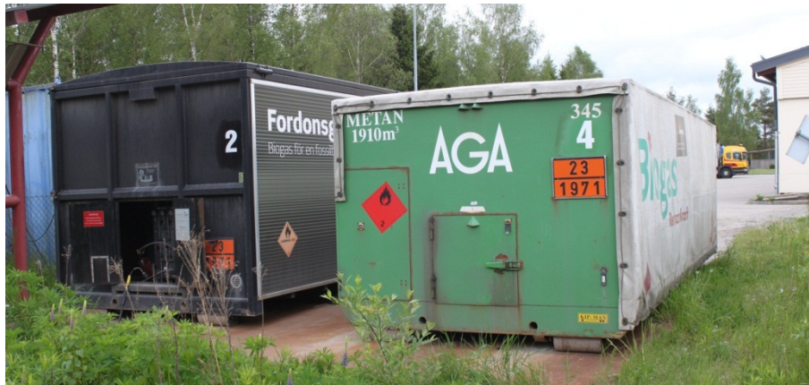
Figure 43: Containers for the transport of CBG of the biogas plant in Borås, Sweden (Source: Rutz)
